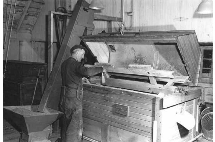
Debrusher - Used to separate seed from stems and seed pods. There was a rotating paddle wheel with brushes fastened to adjustable arms on the wheel and abrasive screen on the sides of the box. Photos courtesy Brian Swaile.
