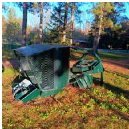
An innovative planting machine with a scarifying wheel.
