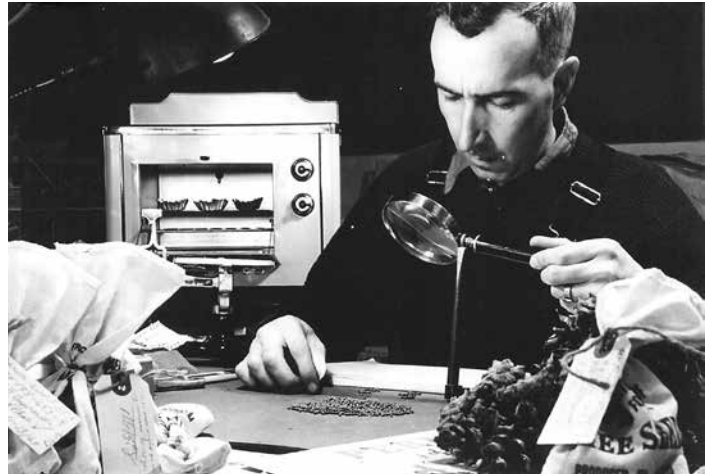
Seed Testing Preparing/counting out seed samples for germination test and also for moisture testing.
